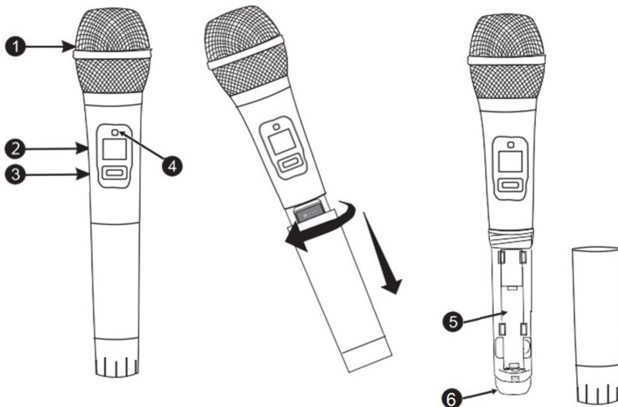
1. Microphone unit and wire mesh cover.
