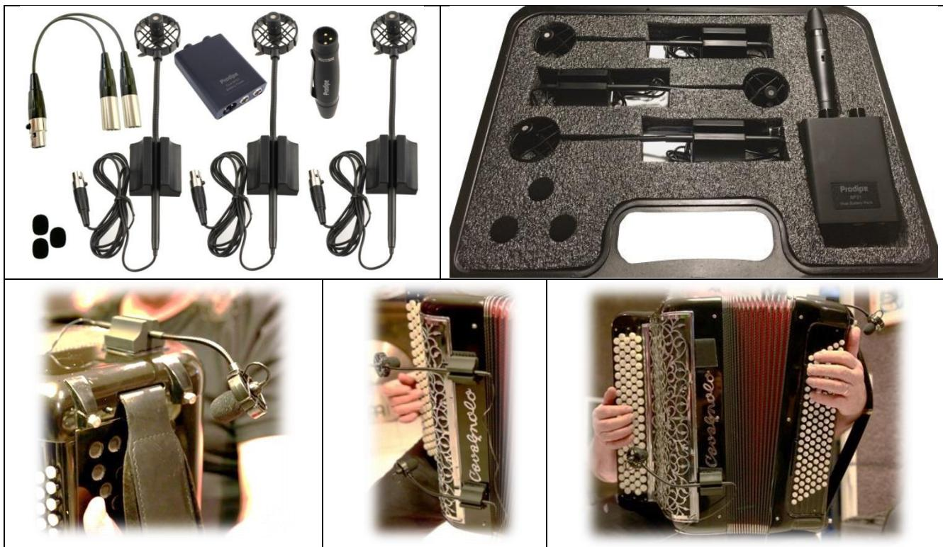
Position the AL21 microphones using the scratch clamps that attach to the accordion, then adjust the proximity of the cells using the goosenecks, by moving the cells closer or further away from the sound outputs of the accordion.
