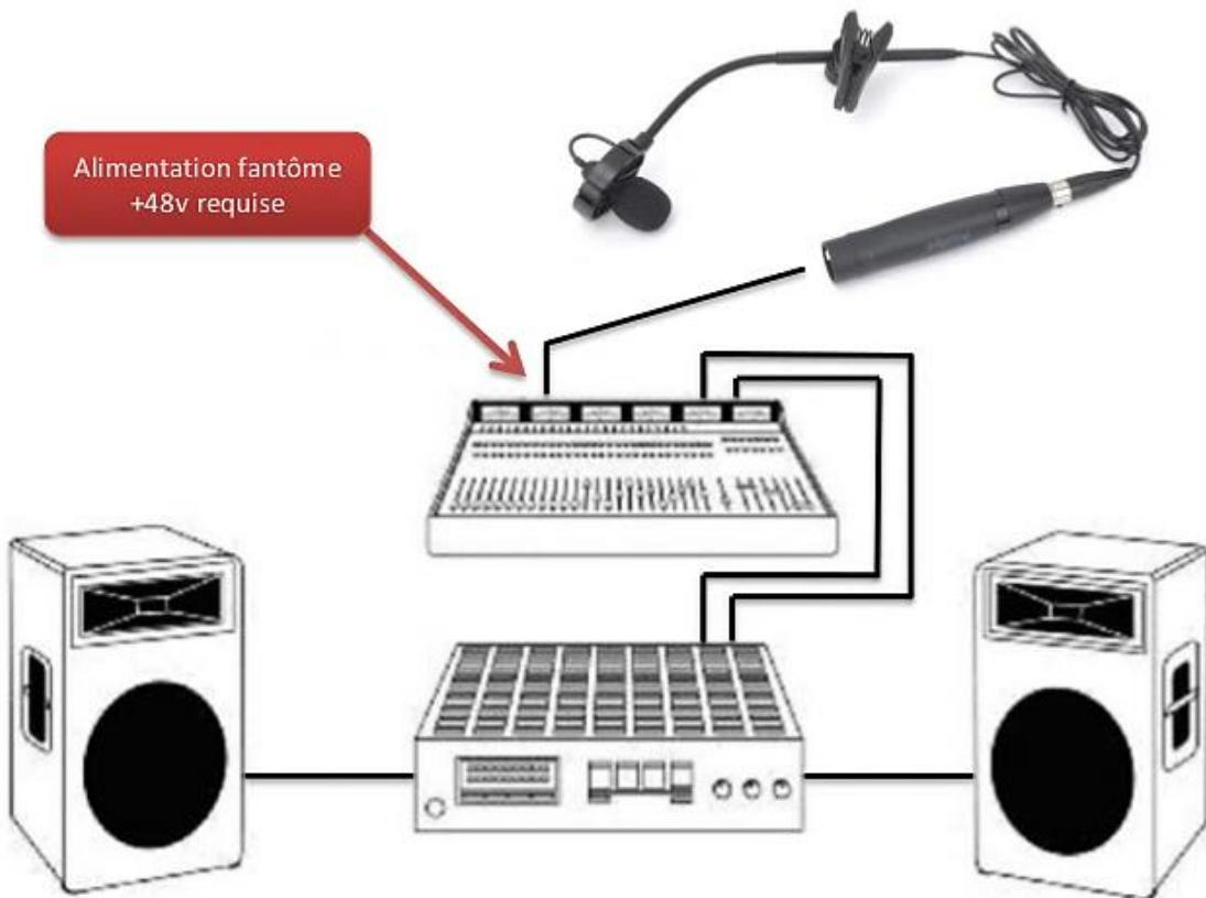
Connect the Lanen Series 21 mic mini XLR socket to the mini XLR to XLR adaptor. Connect your mic with an XLR to XLR cable (not included) to a mixing deck or any other equipment that has an XLR audio input terminal and +48v phantom power.
