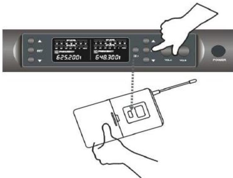
For DSP DUO UHF models with two M850 microphones or two B210 bodypacks you should carry out the same procedure for each microphone or bodypack to synchronize them.
