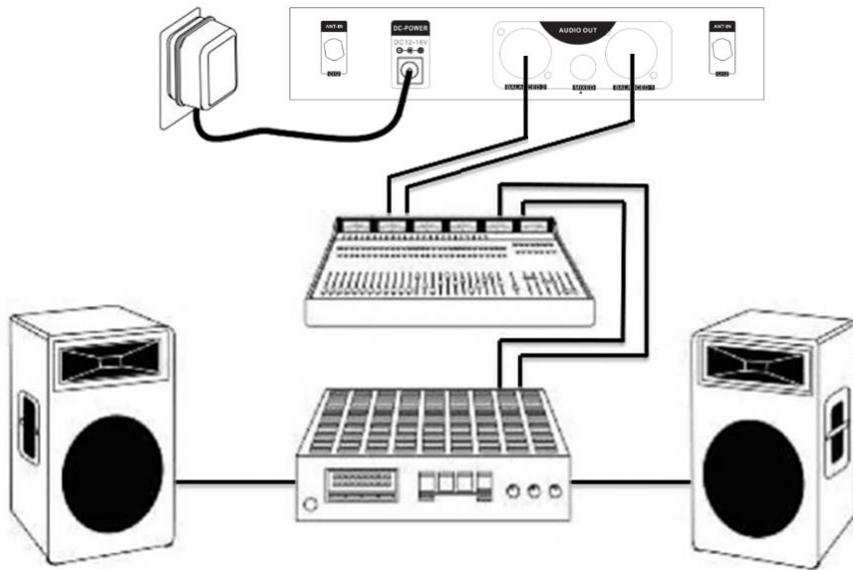
Connect the receiver audio output cable (jack or XLR) to your mixer or broadcasting system.
