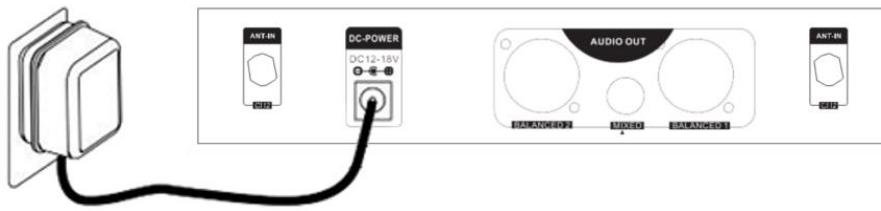
Connect the mains adapter to the socket provided in the back of the receiver and plug into a 230V/50 Hz power source.
