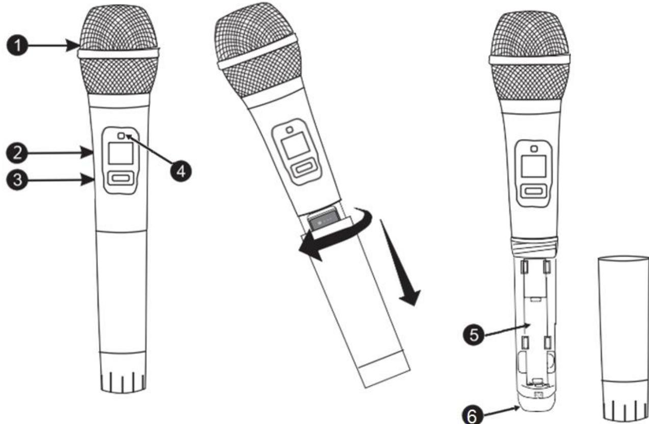
1. Microphone unit and wire mesh cover.
