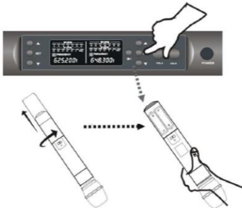
Press the DOWN [▽] button for a few seconds to start the automatic frequency search; once the frequency has been selected, press the [SET] button briefly to validate the frequency, and second press for synchronize the transmitter with the receiver. When the receiver light is green, automatic synchronization is complete.
